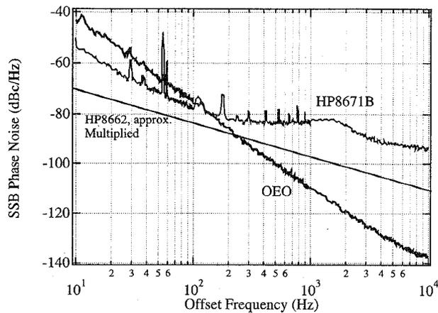
ThT2 Fig. 3. The comparison of the measured phase noise of the dual-loop OEO, the measured phase noise of an HP 8617B synthesizer, and the expected phase noise of an HP8662 synthesizer multiplied to 10 GHz.
