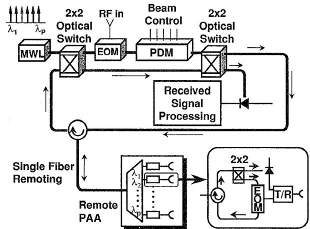
ThT3 Fig. 1. Schematic diagram of the MWOC-PAA T/R module. The transmit and the receive operation are controlled by the  $2 \times 2$  optical switches.
