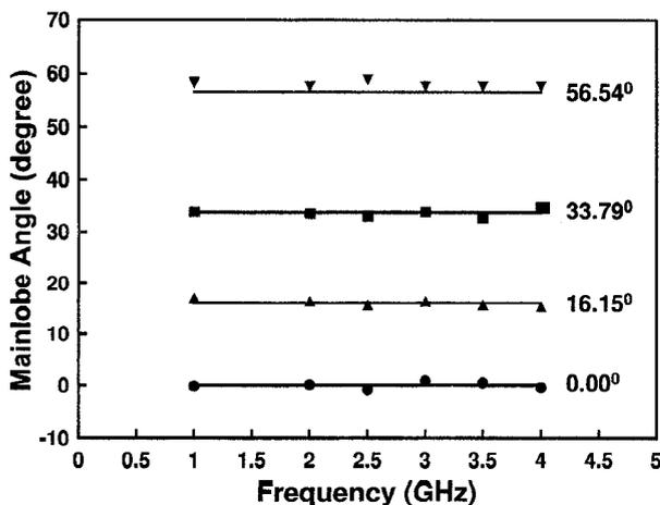
ThT3 Fig. 3. Beam angle vs. microwave frequency for various PDM settings. Squint-free beam receiving is measured up to 4 GHz.
