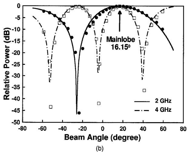
ThT3 Fig. 2. Measured and calculated beam patterns at 2 and 4 GHz. The mainlobe is located at (a) broadside and (b) 16.15°, when a time delay of 0.00 and 97.1 ps, respectively, is generated between the two optical wavelengths by the PDM.
