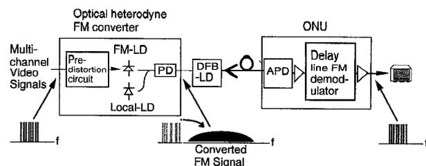
ThT4 Fig. 1. FM converted multichannel video signal transmission system.
